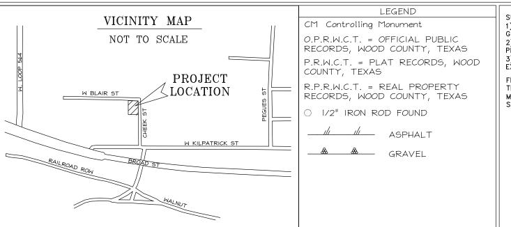
1) BEARINGS ARE BASED ON NAD 83, TEXAS NORTH CENTRAL 4202, AS OBSERVED BY GPS. AREA AND DISTANCES SHOWN HEREON ARE AT GRID. 2) NO EASEMENT RECORD SEARCH WAS MADE BY THIS OFFICE CONCERNING THIS
